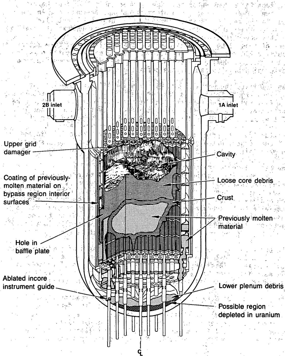
Figure 1. TMI-2 end state core condition.
